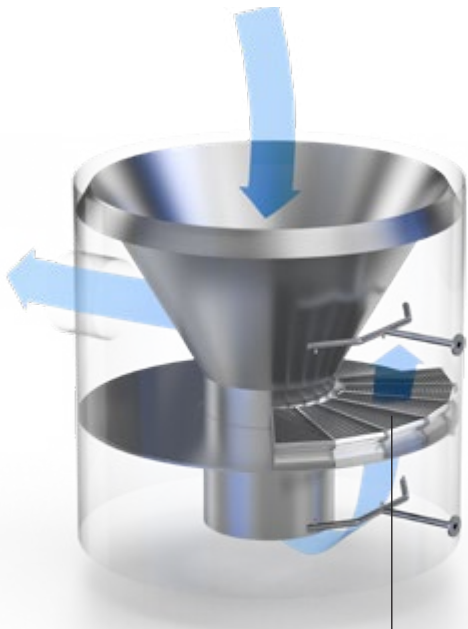
"Cake Piece" separator in an evaporator
