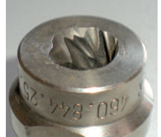
Fig. 2: Wear of a full cone nozzle
