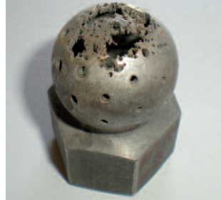
Fig. 1: Chemical corrosion of a spray ball
