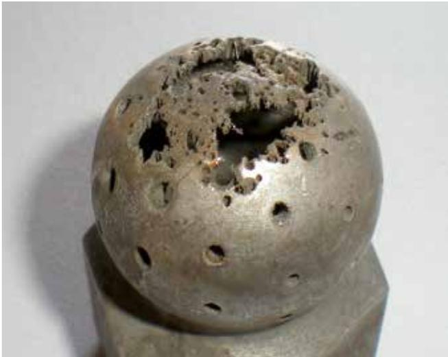
Figure 13: Chemical attack on a spray ball
