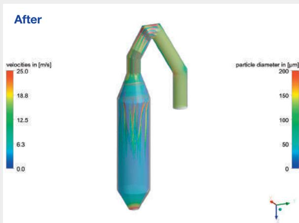
**Optimization of SNCR process – best possible selection and placement of nozzles**
