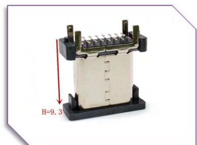
A25-F-V2-H-16 USB Type C 16pin Female Vertical SMT Type
