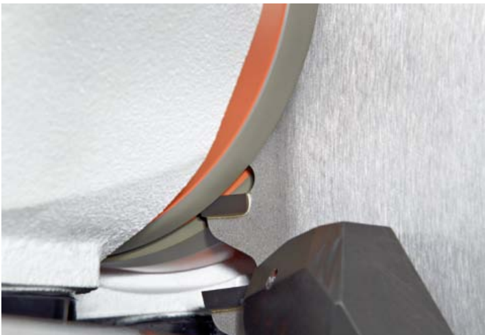
Flat side processing with cup grinding wheel.
