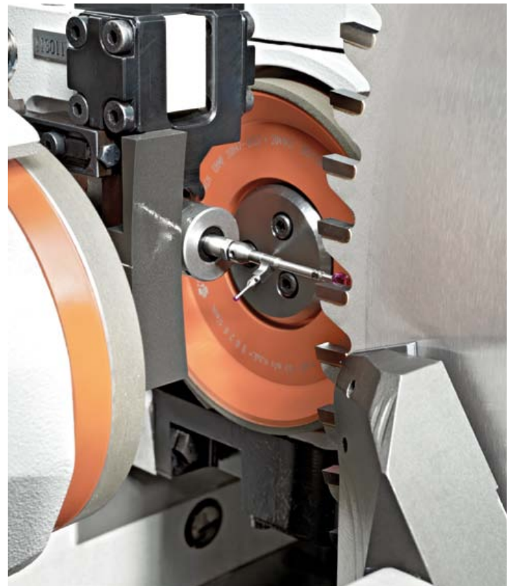
2 main spindles with up to 3 grinding wheels and the centrally situated measuring system.
