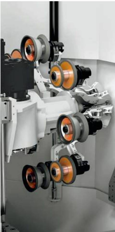
//////// EIGHT-TOOL GRINDING-WHEEL CHANGER for efficient grinding wheel replacement and reduced non-productive time
