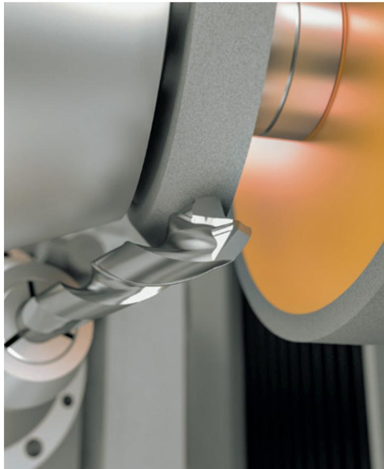
//////// MACHINING CARBIDE DRILLS
