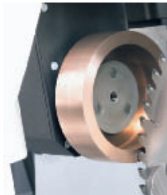
Working position of the rotary electrode at the circumference of the saw blade
