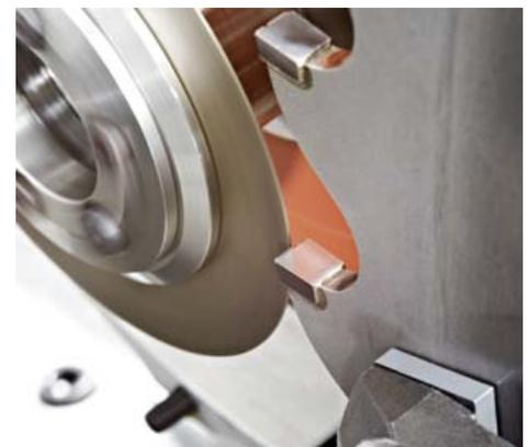
Grinding of chip breaker groove.
