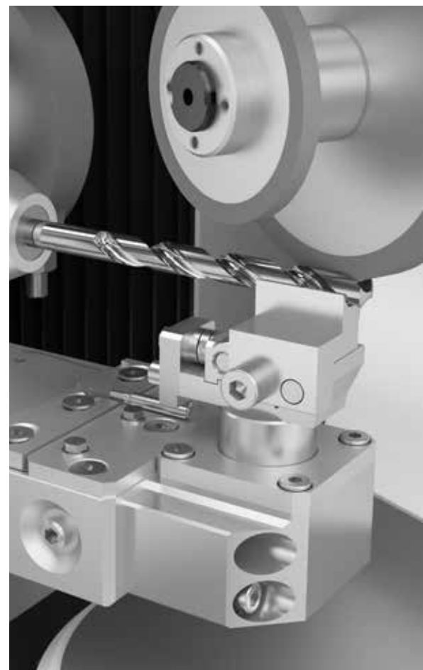
///// STEADY REST WITH AUTOMATIC STROKE ensures an optimal grinding result for longer tools
