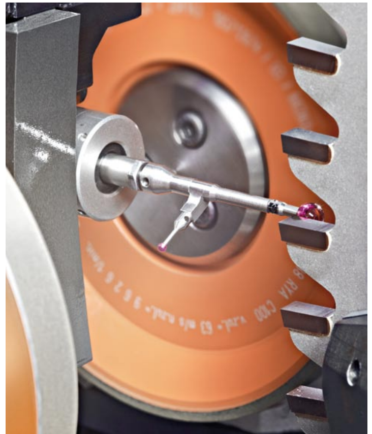
The measuring probe, which is standard equipment within the machine, takes all relevant parameters such as saw blade diameter, hook angle, width of saw blade body, tooth side projection, and side clearance angle.
