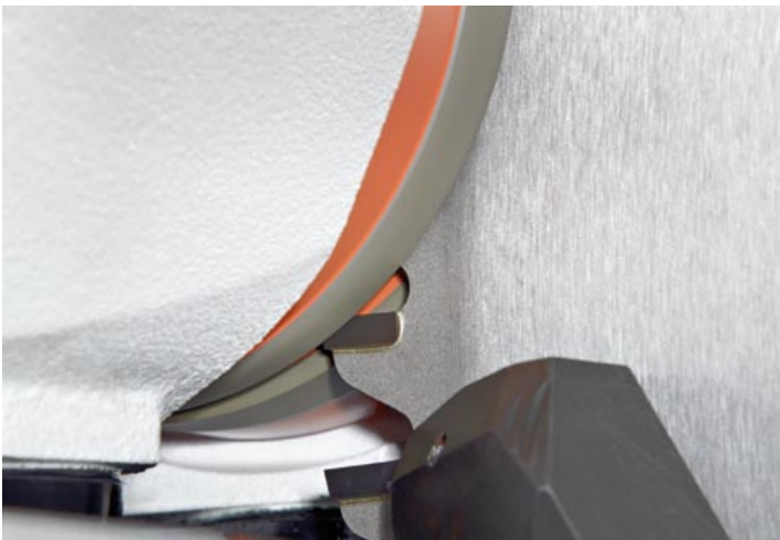
Flat side processing with cup grinding wheel.
