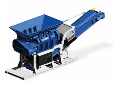
Hopper Capacity: 3.80 m<sup>3</sup> Length: 3.50 m Width: 2.00 m
