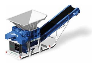
**Hopper** Capacity: 3.00 m<sup>3</sup> Length: 3.00 m Width: 2.00 m
