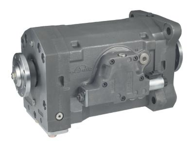
This new axial piston motor has been developed by Linde Hydraulics to achieve maximum speeds higher than conventional swash plate designs. Additionally, a large displacement volume in a compact design means wider transmission speed ranges, normally achieved with modular transmissions, are possible. The HMV-02 D is about 30 % lighter than a motor combined with transfer gear box, and has a smaller footprint.
