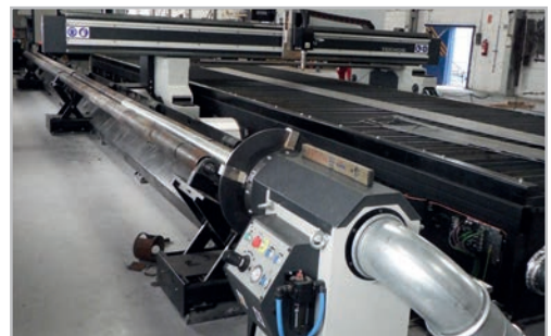
Tube cutting with servo-controlled rotation Corte de tubos con giro servo-controlado
