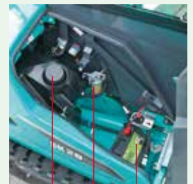
Fuel tank Battery Water separator
