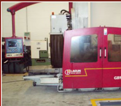
FRESADORA LAGUN GBM-18 , mesa 1.800x700, long. 1.700, Trans. 800, vert. 800, ISO-50, 23 cv, Control Fagor 8055
