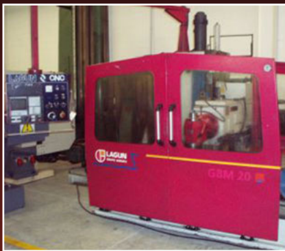
FRESADORA LAGUN GBM-20 , mesa 2.000x750, long. 1.8300, Trans. 940, vert. 1.000, ISO-50, 27 cv, Control Fagor 8025M
