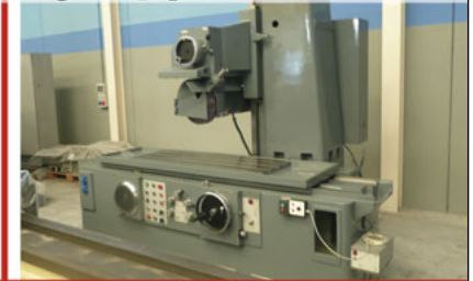
Rectificadora DANOBAT RT1200 Long. 1.200 mm, anchura 550 mm. Mesa 1.200 x 450
