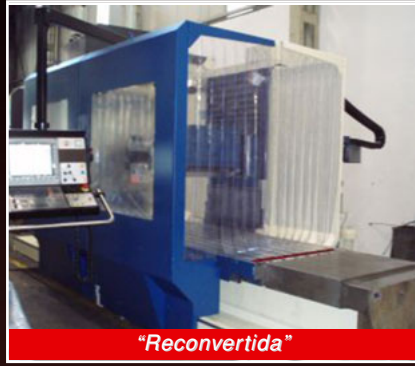
FRESADORA CORREA A-25/25 , mesa 2.800x900, long. 2.500, Trans. 1.000, vert. 1.000, ISO-50, 25 cv, Control Heidenhain TNC-530
