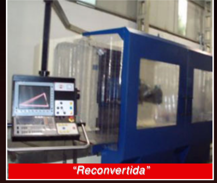
FRESADORA CORREA A-25/30 , mesa 3.500x1.100, long. 3.000, Trans. 1.200, vert. 1.000, ISO-50, 30 cv, Control Heidenhain TNC-530
