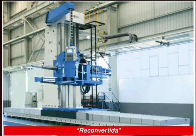
MANDRINADORA WOTAN B-160P, Ø 160, mesa 1.800x2.100, long. 1.300, Trans. 6.000, vert. 2.500, 40 cv, control Heidenhain TNC-530
