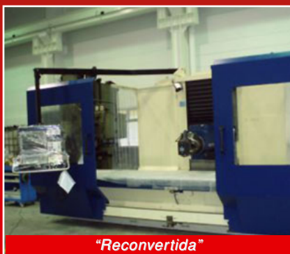
FRESADORA CORREA A-25/30 , mesa 3.500x1.000, long. 3.000, Trans. 1.200, vert. 1.000, ISO-50, 30 cv, Control Fagor 8050M
