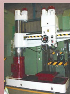
Taladro Radial STANKOIMPORT Ø 55mm
