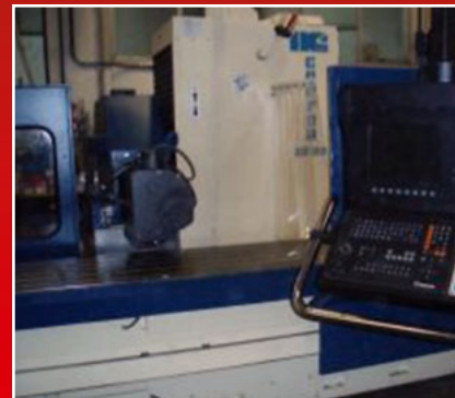
FRESADORA CORREA CF-22/25 , mesa 2.500x700, long. 2.500, Trans. 800, vert. 800, ISO-50, 30 cv, Control Heidenhain TNC-407
