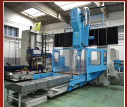
FRESADORA ZAYER KP-4000 , mesa 4.000x1.800, long. 3.700, Trans. 3.050, vert. 1.100, ISO-50, 49 cv, Control Heidenhain TNC-430M
