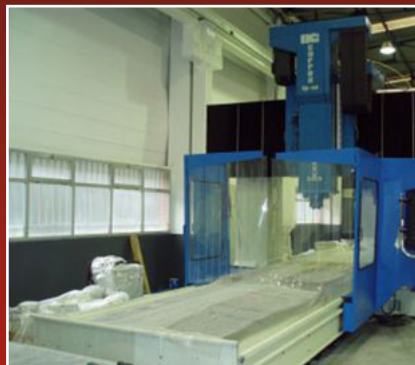
FRESADORA CORREA FP-40/40 , mesa 4.000x1.250, long. 3.500, Trans. 2.500, vert. 1.000, ISO-50, 30 cv, Control Heidenhain TNC-407A
