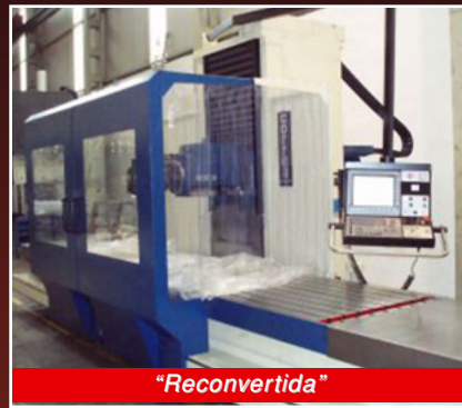
FRESADORA CORREA A-25/50 , mesa 5.000x1.000, long. 5.500, Trans. 1.200, vert. 1.500, ISO-50, 25 cv, Control Heidenhain TNC-530
