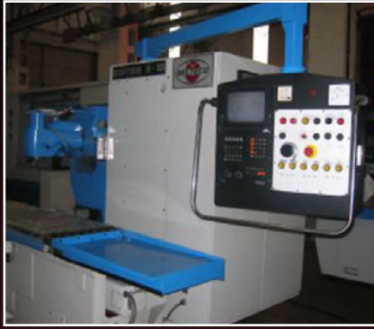
FRESADORA CORREA A-10 , mesa 1.700x560, long. 1.300, Trans. 630, vert. 630, ISO-50, 12 cv, Control Heidenhain TNC-150
